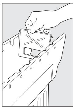
**STEP 5** Install Rear Door of Newspaper Port by snapping pegs into the back indentations of the Newspaper port. Installing the mailbox will create a tight hold on the rear door.
