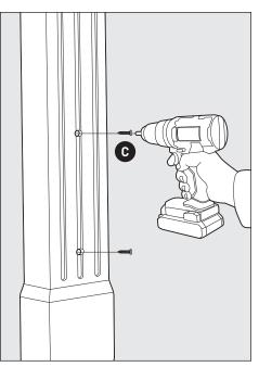
**STEP 3** Secure the Mailbox Post Sleeve section to the 4x4 treated pine post using the (4) #12 x 1" screws **③** included in the kit. Screws will go through the plastic with slight pressure. Do not over tighten.
