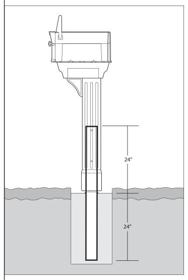
**STEP 1** Determine location for mailbox. Using post hole digger, dig a hole 24" in depth. Install treated pine post by burying 24" of the post in the ground - leaving at least 24" of post above ground. Use level to ensure treated pine post is in correct vertical position. Stabilize the treated pine post by firmly tamping down loose soil around post base.
