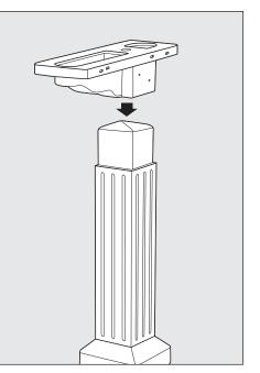
**STEP 4** Attach Mounting Bracket to top of Mailbox Post Sleeve.
