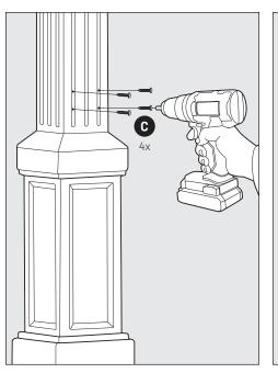
**STEP 3** Secure the Mailbox Post Sleeve section to the 4x4 treated pine post using the (4) #12 x 1" screws ③ included in the kit. The Plastic post has (4) Mounting Holes located approximately 23 inches above bottom of post.
