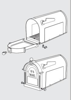
**STEP 6** Assemble your mailbox by using (2) pins to attach Mailbox Door to holes in Mailbox Body. Pins can be snapped into place by pressing firmly with thumb or tapped in using a rubber mallet. **TIP:** Make sure the pins are fully snapped into place. If they are installed correctly, you will not be able to remove the pins with your fingers.
