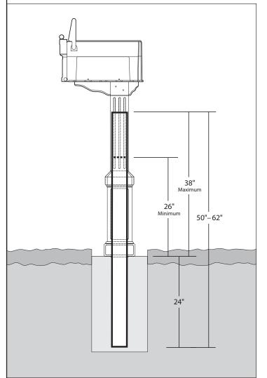
**STEP 1** Determine location for mailbox. Using post hole digger, dig a hole 24" in depth. Install treated pine post by burying 24" of the post in the ground - leaving at least 26" of post above ground. The 4x4 post can be up to 38" above ground, but only 26" is necessary. Use level to ensure treated pine post is in correct vertical position. Stabilize the treated pine post by firmly tamping down loose soil around post base.
