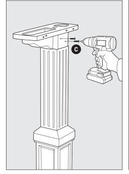
**STEP 5** Using the (4) #12 x 1" screws **(b)** secure the Mounting Bracket to the Post Sleeve. Do not over tighten screws.
