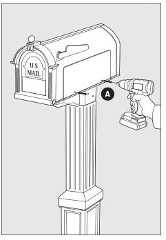
**STEP 7** Place Mailbox on to top of Mailbox Post Bracket, align holes of mailbox & bracket and secure with (4) 24 x 1-1/2" Phillips Machine Bolts (A) and nuts (B).
