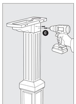
**STEP 5** Using the (4) #12 x 1" screws **©** secure the Mounting Bracket to the Post Sleeve. Do not over tighten screws.
