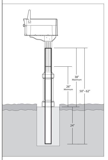
**STEP 1** Determine location for mailbox. Using post hole digger, dig a hole 24" in depth. Install treated pine post by burying 24" of the post in the ground - leaving at least 26" of post above ground. The 4x4 post can be up to 38" above ground, but only 26" is necessary. Use level to ensure treated pine post is in correct vertical position. Stabilize the treated pine post by firmly tamping down loose soil around post base.
