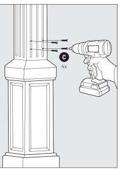
**STEP 3** Secure the Mailbox Post Sleeve section to the 4x4 treated pine post using the (4) #12 x 1" screws **②** included in the kit. The Plastic post has (4) Mounting Holes located approximately 23 inches above bottom of post.
