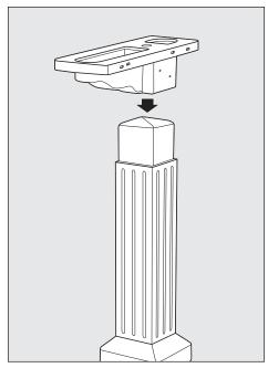
**STEP 4** Attach Mounting Bracket to top of Mailbox Post Sleeve.
