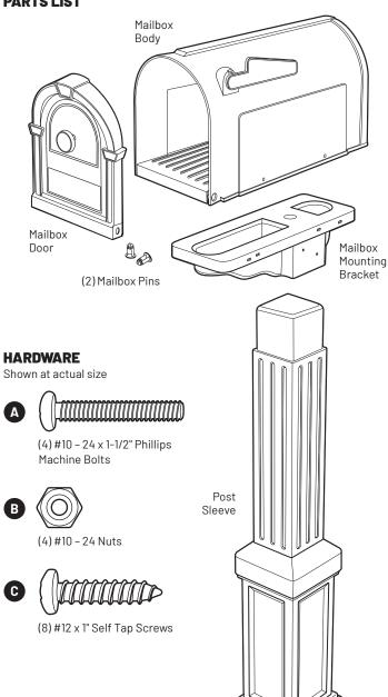
NOTE: Customers are required to contact the local post office before installing the mailbox to ensure its correct placement and height at the street. Generally, mailboxes are installed at the height of 41–45 inches from the road surface to inside floor of mailbox or point of mail entry (locked designs) and are set back 6–8 inches from front face of curb or road edge to the mailbox door.
